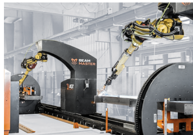
AUTOMATED BEAM WELDING
